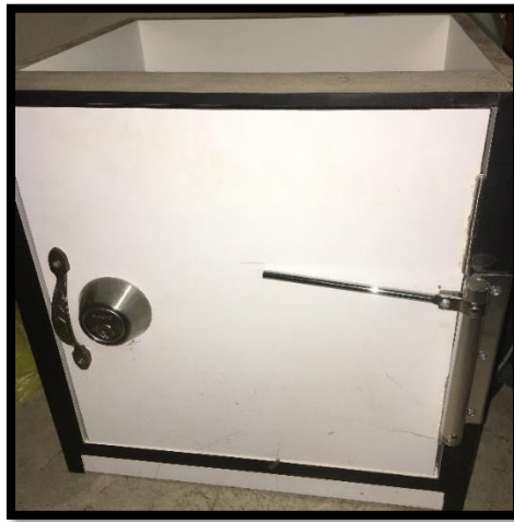
Figure 6: Installation of Automatic Door Closer
