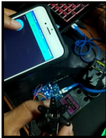
Figure 20: Test run servo motor through Blynk application
